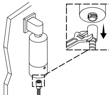
**2** Twist the filter housing cap counterclockwise to remove.
