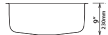
KBU12 23" x 17 1/2" x 9" Min Cabinet Size: 27" Matching Grid: KBG-12 Drain Model #: BST-1
