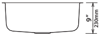
KBU10 23 3/8" x 21" x 9" Min Cabinet Size: 27" Matching Grid: KBG-10 Drain Model #: BST-1
