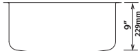
KBU11 20 3/4" x 17 3/4" x 9" Min Cabinet Size: 24" Matching Grid: KBG-11 Drain Model #: BST-1
