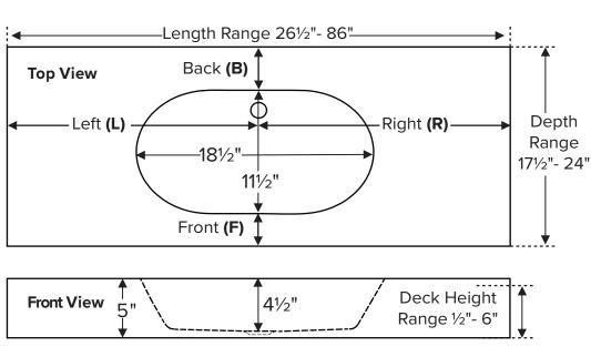
**NOTE:** Counter-sinks with a length of 36" and under have a maximum depth of 23".
