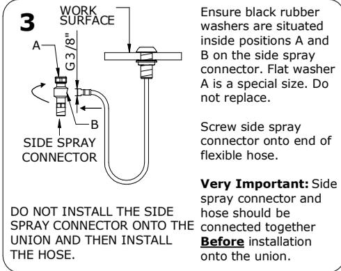
Ensure black rubber washers are situated inside positions A and B on the side spray connector. Flat washer A is a special size. Do not replace.
